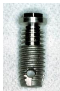
Fig. 1: Prototype of the Hybrid Implant concept from 1993. Published in Ref. 1.
